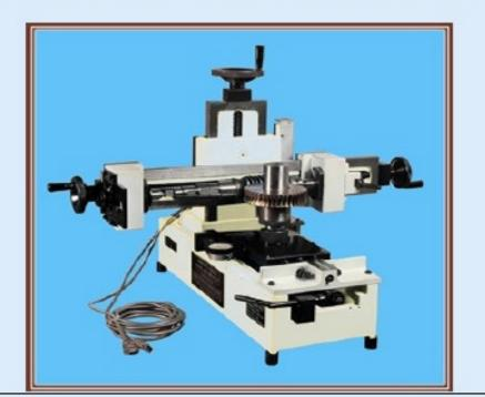
**Cluster Shaft Gear Roll tester**
